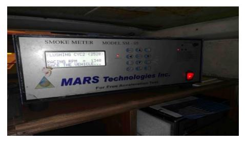
Figure 6: Emissions testing equipment: Smoke Meter Model SM 05; Acceleration tests provided by Mars Technologies Inc
