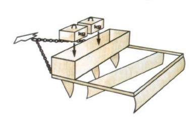
Beam Drag rolled steel joists) or steel rail(s), weighted with concrete blocks, and towed at an angle to the road.
