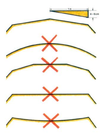
The aim should be to develop a proper **crown\*** on the road.
