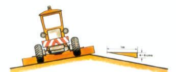
m The material is alternately spread by the grader and watered with the tanker until its moisture content is correct for compaction\*.
