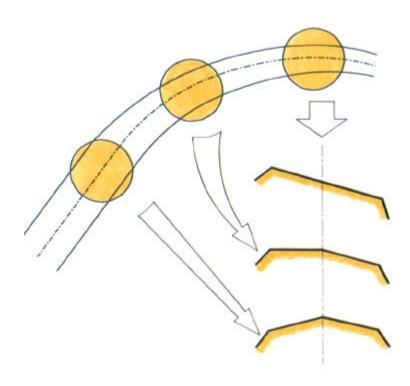
The superelevation must be retained for the complete length of the bend.
