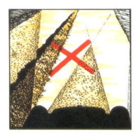
Do not make a final pass down the centre of the road with the grader blade horizontal.
