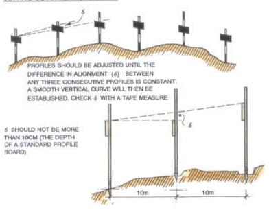
WHEN THE CURVE IS ACCEPTABLE, PLACE NEW CENTRE UNE PEGS AT EACH RANGING ROD WITH TOPS AT 1m BELOW THE PROFILE BOARDS - THIS IS THE FINISHED ROAD CENTRE LINE LEVEL
