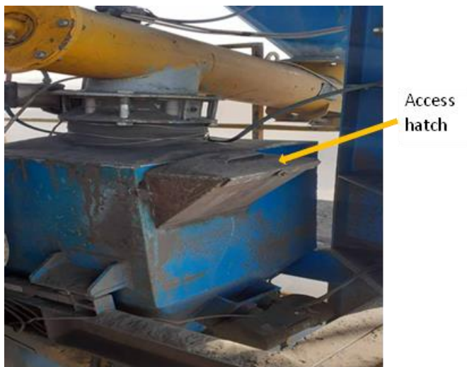
Figure 13 Location of hatch through which fibre and Portland cement were added to the pugmill
