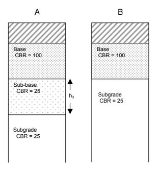
Figure 1 Identical pavements, different structural numbers
