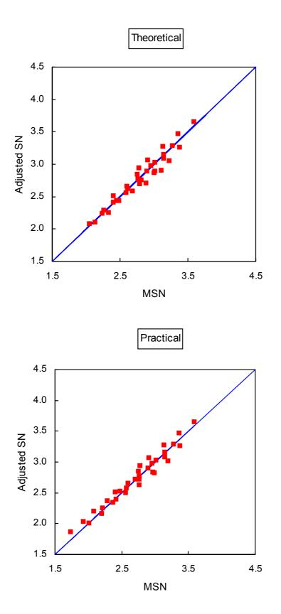
Figure 2. Comparison of the new adjusted method to the original method for typical pavement structures (Road Note 31 Chart 1)
