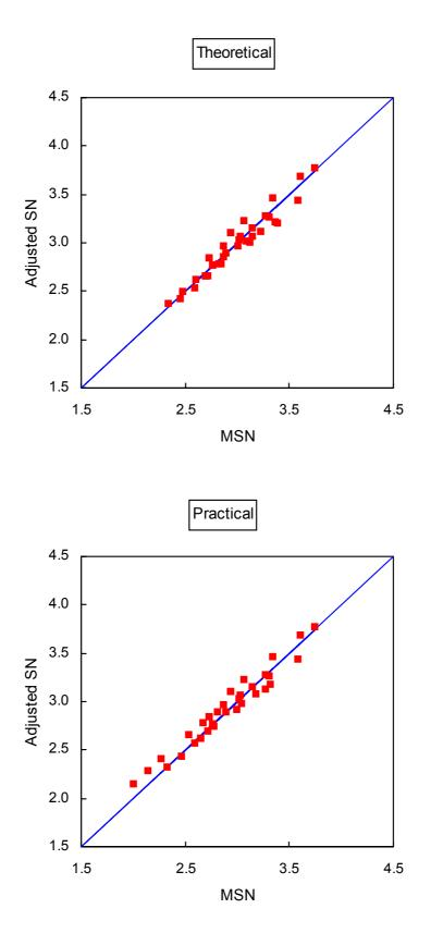
Figure 3. Comparison of the new adjusted method to the original method for typical pavement structures (Road Note 31 Chart 8)
