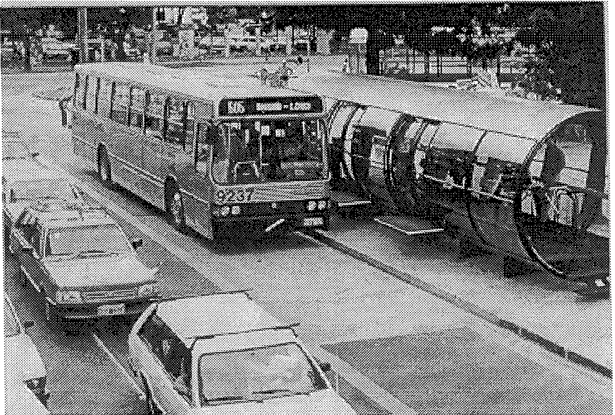
Plate 3: A bus stop on a lane reserved for buses only. Curitiba, Brazil
