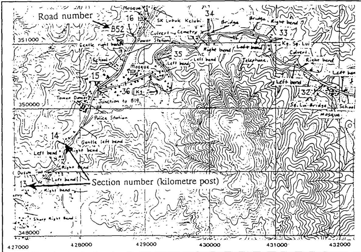
Fig. 11 Example of 1:25000 landmark map for rural roads
