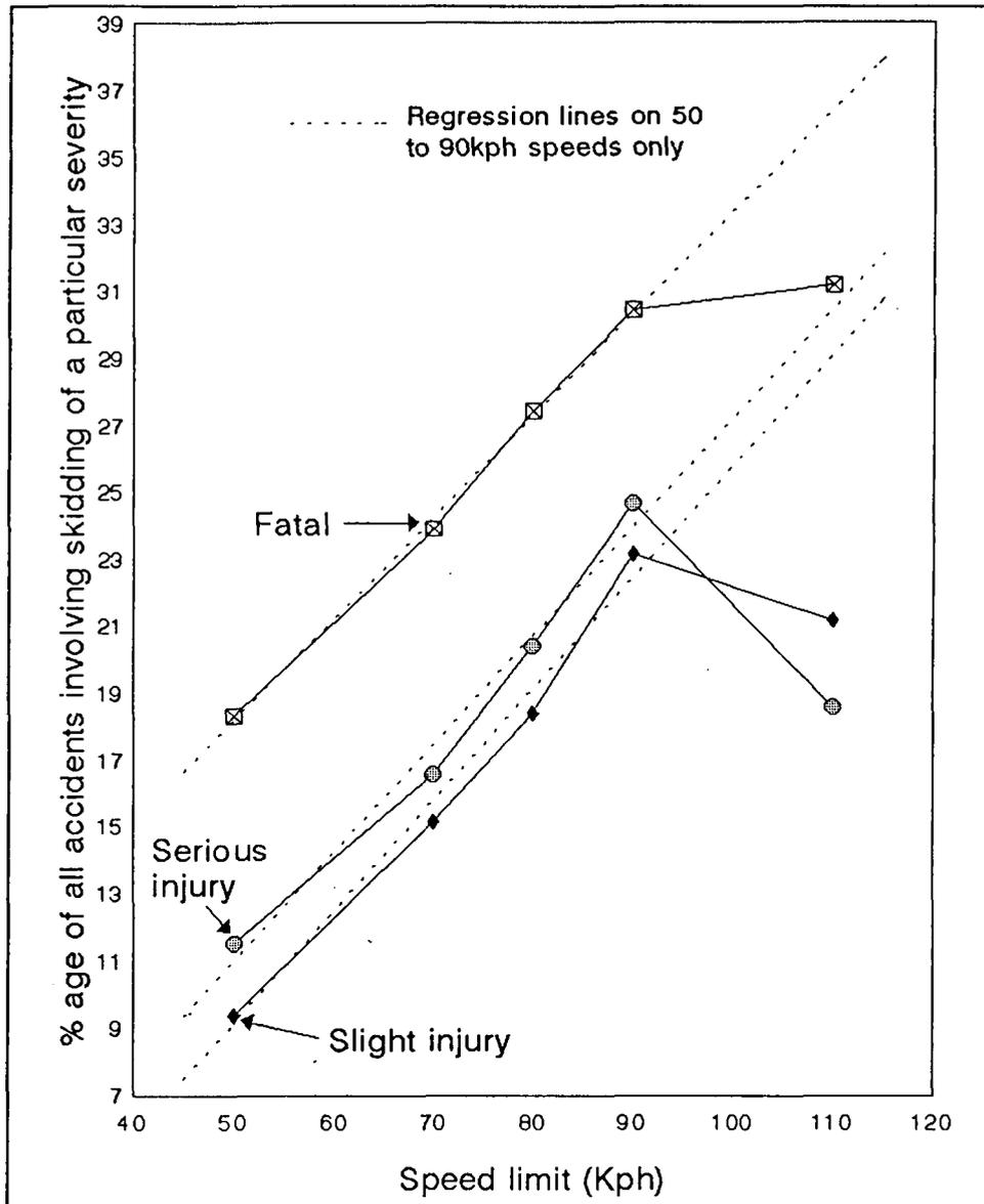
Fig. 9 Accidents involving skidding as a percentage of all accidents of given severity
