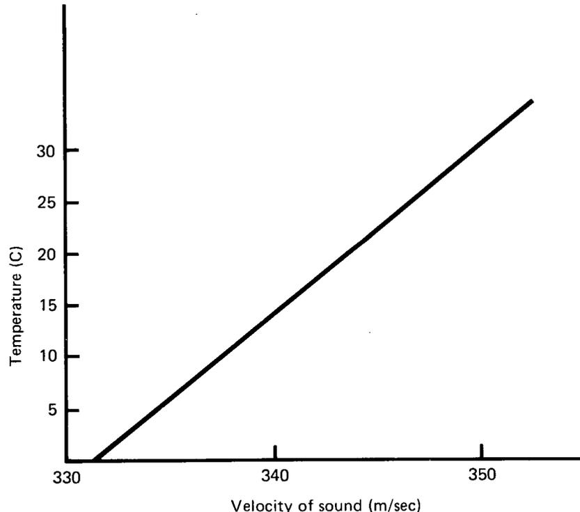
Figure 2. Variations in the velocity of sound with temperature
