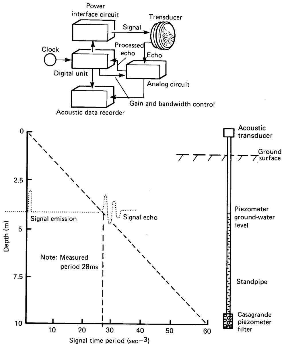
Figure 3. General details of the acoustic method of piezometer monitoring
