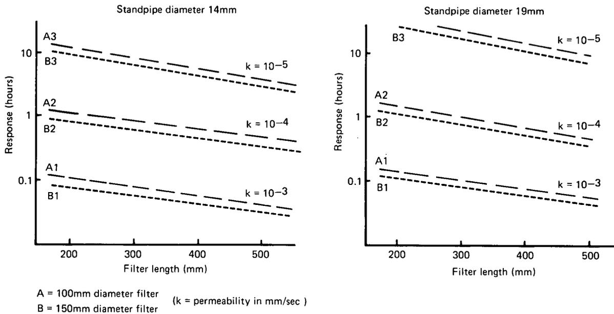
Figure 1. Time lag response curves for 90 per cent equalization calculated from the Hvorslev equation
