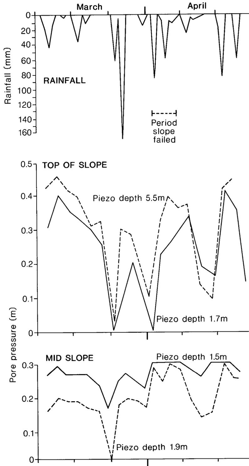
Figure 6. Pore pressure data recorded by the acoustic system for the top of slope (location P1 figure 5) and mid slope (P2) sites in relation to site rainfall
