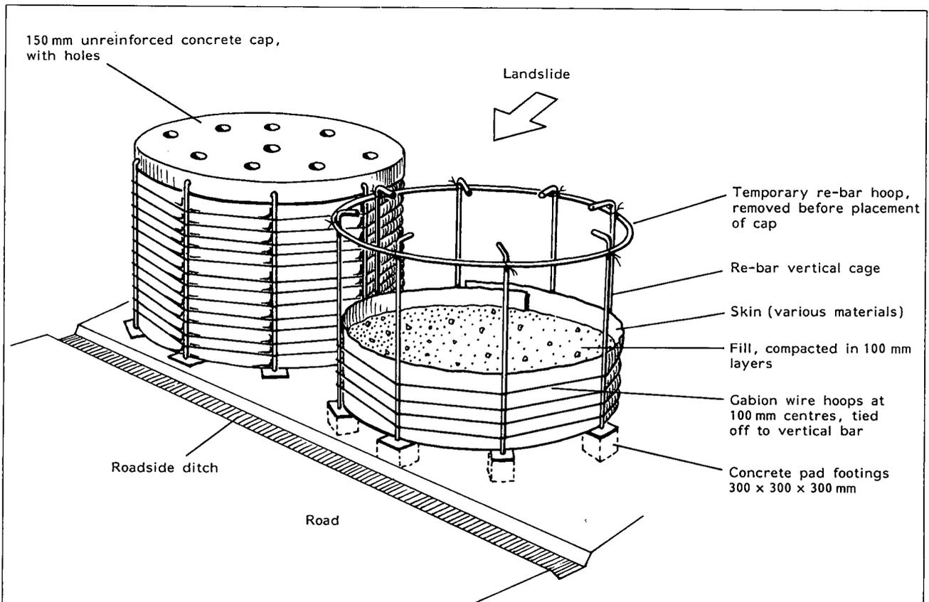
Fig 4 Schematic drawing of cylinder design and method of construction. The skin and fill are placed in lifts. In the revised design the structural concrete cap was replaced by a masonry weather capping
