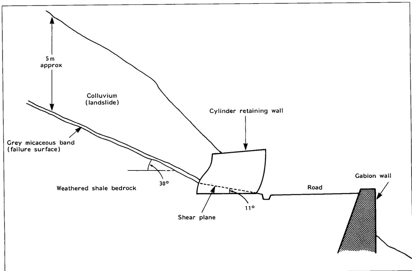
Fig 6 Section through landslide and cylinder wall with unstabilized fill
