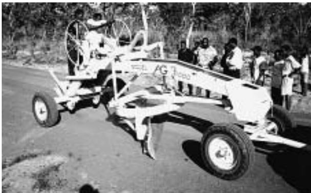
This locally manufactured grader is towed by a tractor and can be used for formation works and for maintaining earth and gravel surfaces.
