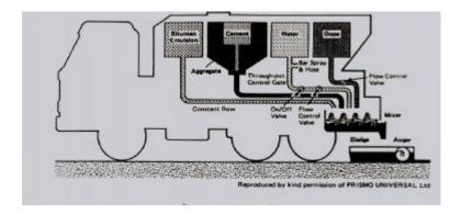
Slurry seal machine; (diagrammatic)
