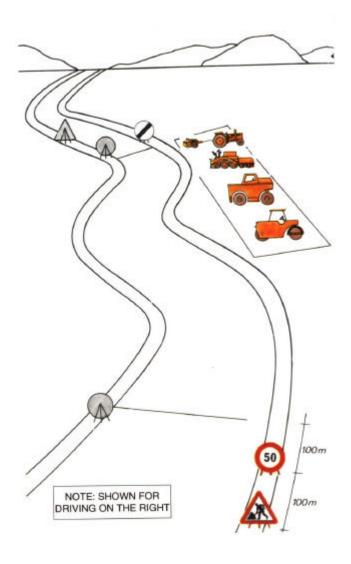
At the end of each day, the road is opened to traffic, but the following signs must be retained at the ends of the new section:
