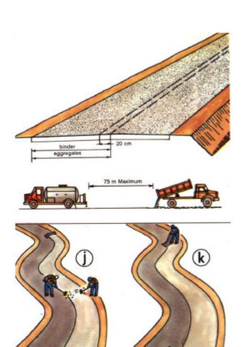
for the second half-width of the road, aggregate is spread over the remaining width of the binder including the strip left un-covered.
