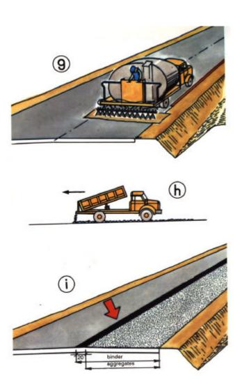
The distributor jets are opened over the first strip of paper and closed over the strip at the end of the run **(g)**.
