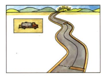
**4 Place strips of strong paper in position** to ensure regular transverse joints at the beginning and end of each pass of the distributor.
