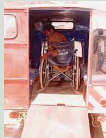
*Figure 3.51 Side and rear view of a 3-wheeled motorcycle turned into a prototype accessible van (Courtesy of Wycliffe Kepha)*
