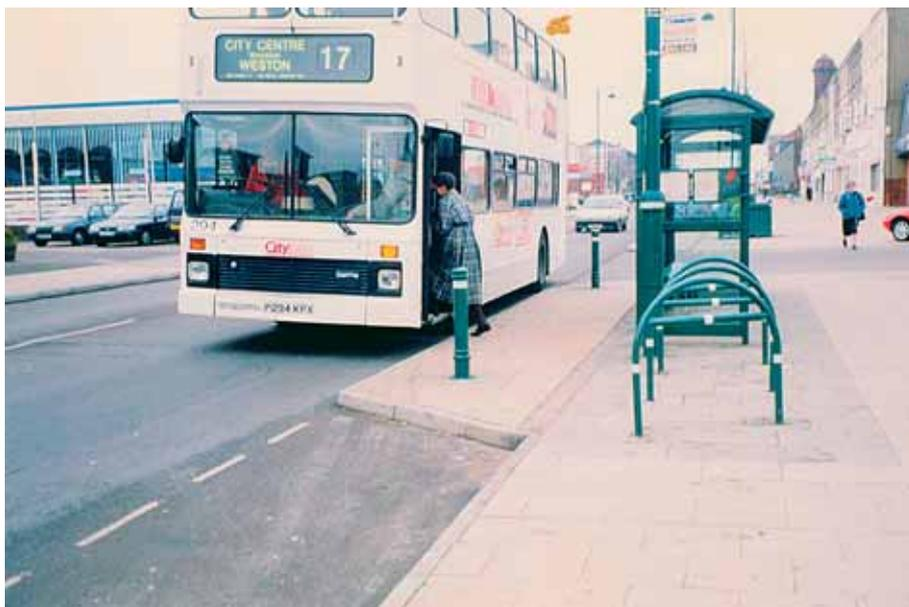
**Figure 3.24** A bus bulb or boarder in operation
