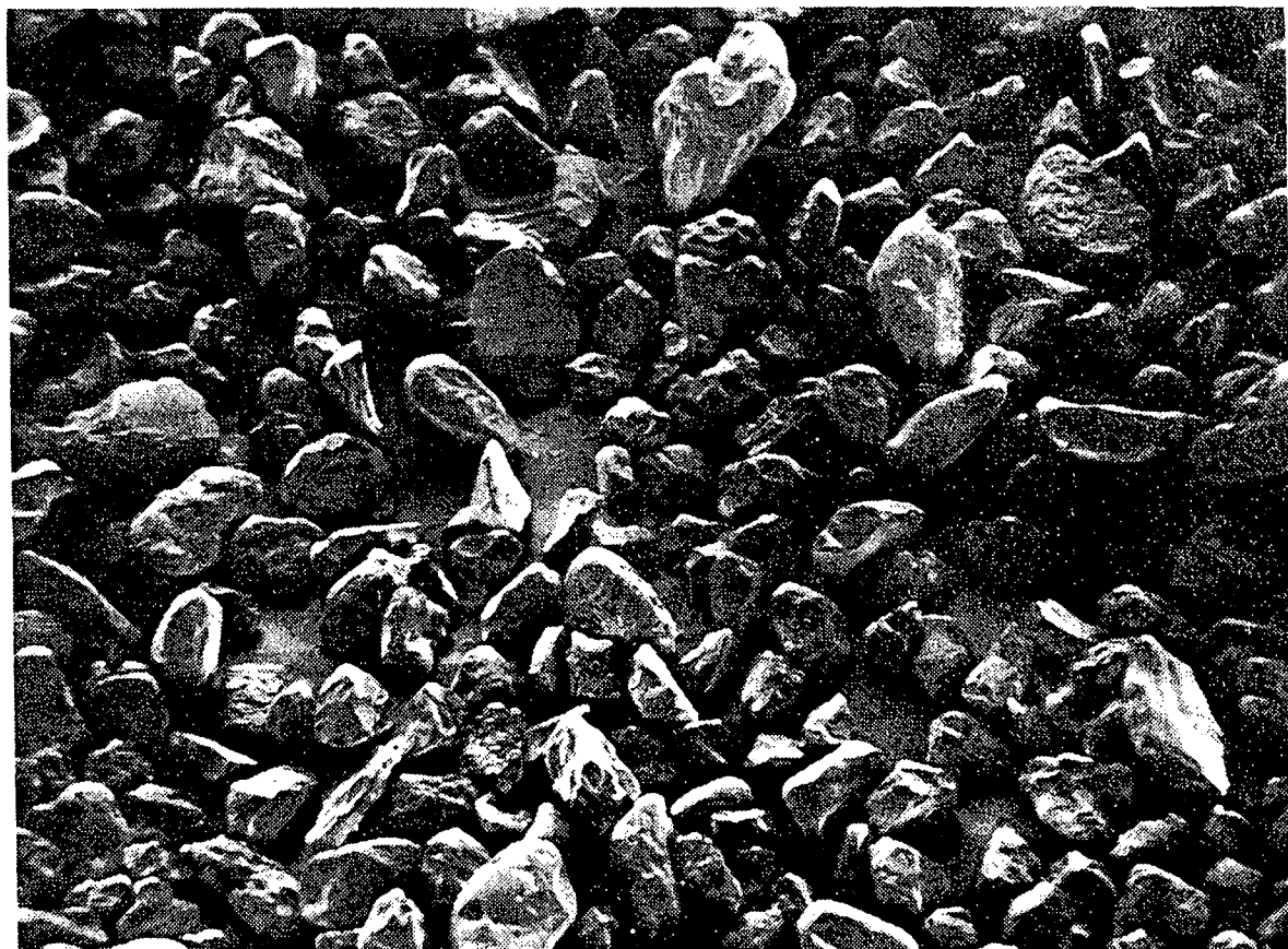
Fig. 4. Damaturu-Baiomori road; electron-photomicrograph of sand fraction 210-75 μm
