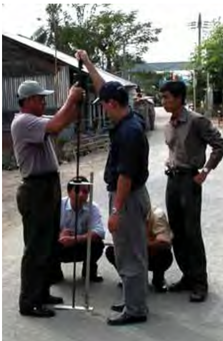
Figure 9.7: Dynamic cone penetrometer in use for measuring the strength of an existing pavement
