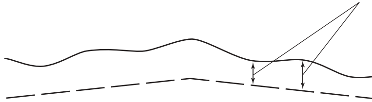
2. Measurement of gravel thickness on deteriorated road with four wheelpaths
