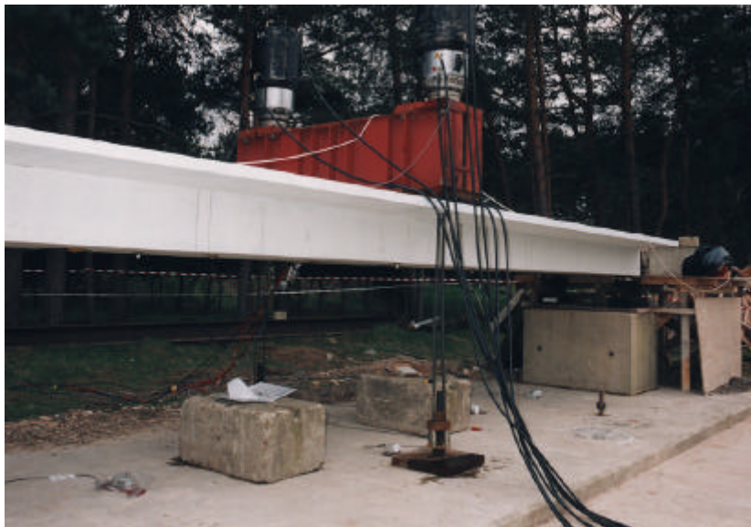
Figure 5 Model bridge ready for load test.
