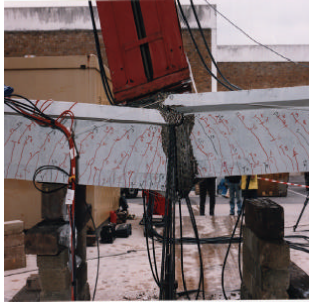
Figure 7 Failed model after load test 1.
