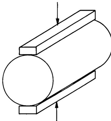
Fig.4 THE INDIRECT TENSILE TEST
