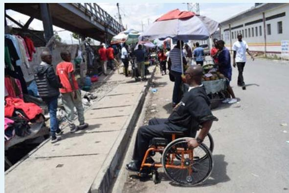
Image above: A footway at a different height to the street, with no ramp prevents the man in a wheelchair from joining the footway in Kenya.
