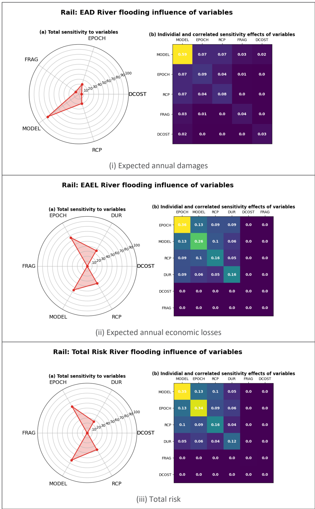
Figure A 19: Influence of variables on different risk parameters for river flooding of railways
