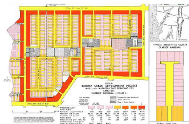
Figure 33: Site plan at Charkop showing the grid pattern of roads
