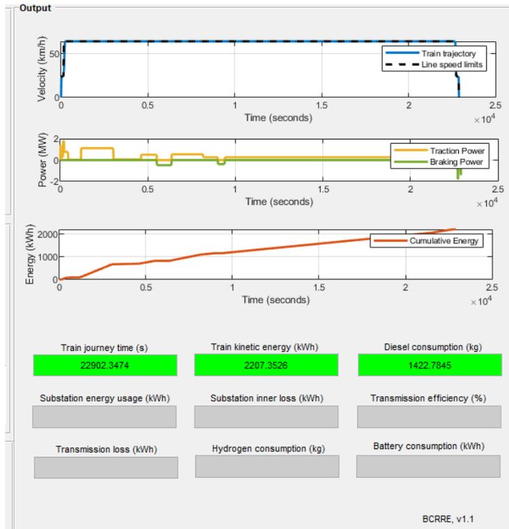
Figure B.4: Simulation output for the Tabora – Mwanza section, using the diesel only train
