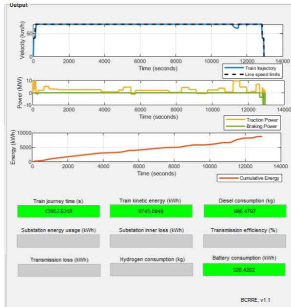
Figure 26 shows the simulator outputs for a loaded diesel-hybrid train from Tokadeh -Buchanan.
