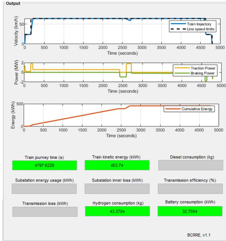
Note that the hybrid battery charge declines by 15% in Figure B.7.
