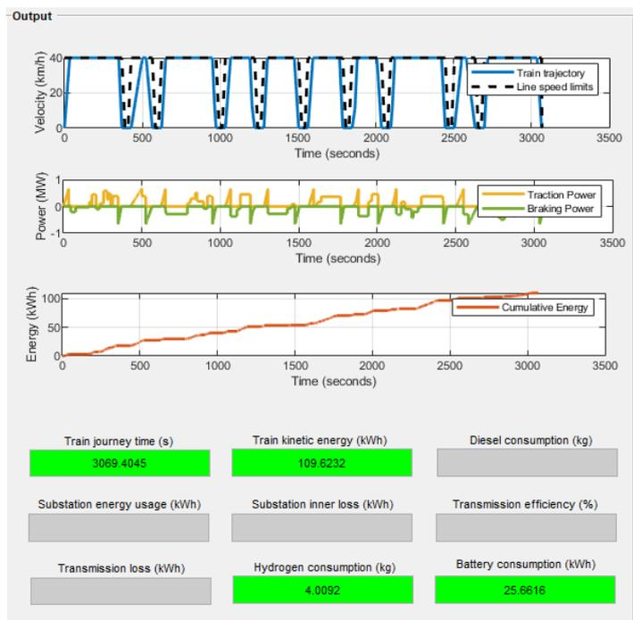
Figure 14: Simulation output for the Kampala – Namanve route, using the diesel hybrid ULR-based train
