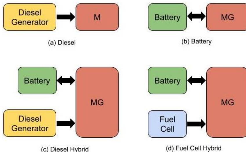
Each of the architectures shown either uses a fuel to generate electricity, and/or has an on-board store of electricity (i.e. a battery) to power or help power the train. In the case of Figure(a), the electric motor is used to purely power the train, but in the case of Figure(b), (c) and (d) the electric motor can also be used as a generator to help slow the train down while generating electricity that can then be stored using on-board batteries for later reuse (i.e. a ‘Motor Generator’).
