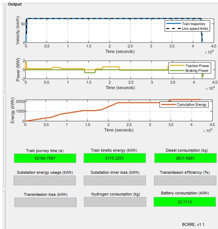
Note that the hybrid battery charge declines by 15% in Figure B.13.
