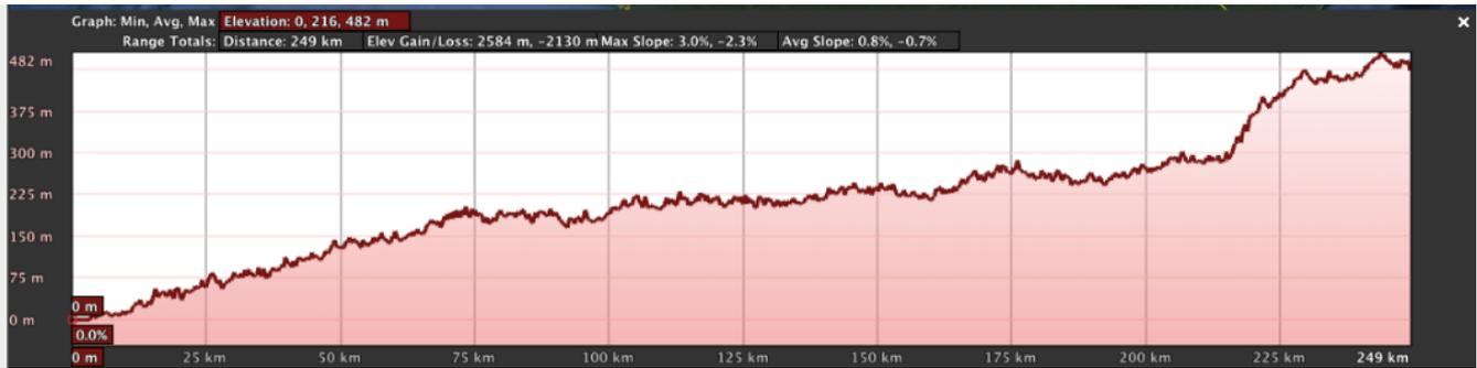
As this route is far longer than the Kampala line, it was not modelled in a great level of detail; with altitude assessed at roughly 2 km intervals to give the route profile shown in Figure 19.
