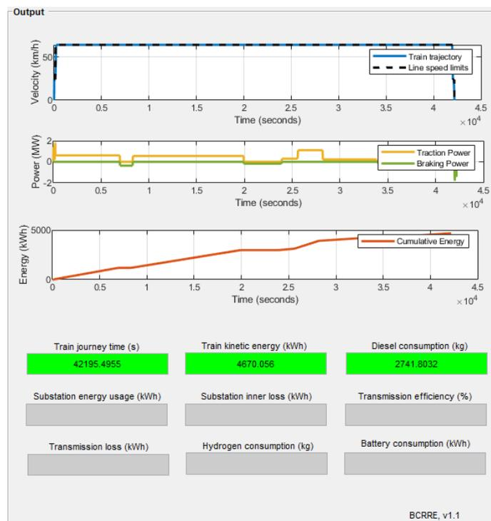
Figure B.3: Simulation output for the Kigoma – Tabora section, using the diesel only train
