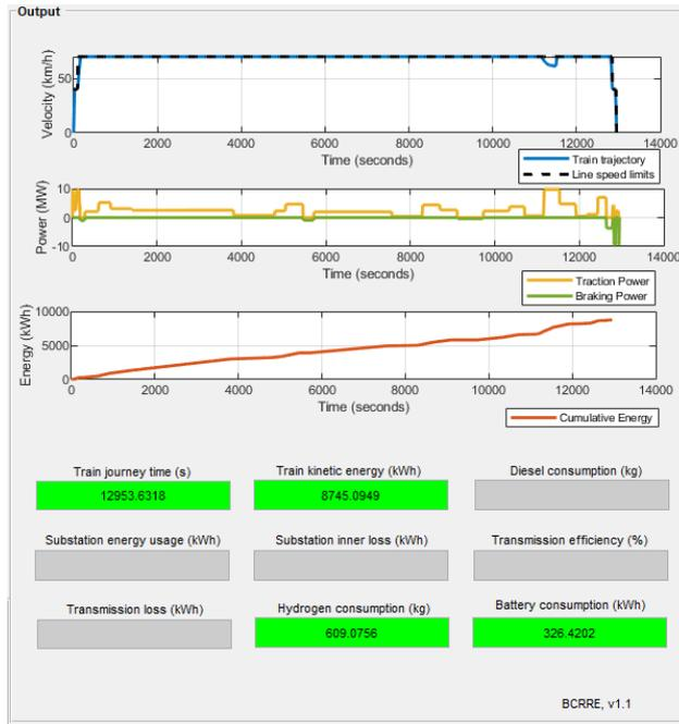
Figure 24 shows the simulator outputs for a loaded hydrogen-hybrid train from Tokadeh -Buchanan.
