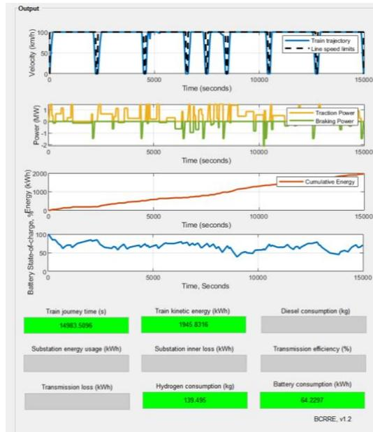
Figure 47 shows the simulator outputs for the diesel hybrid train.
