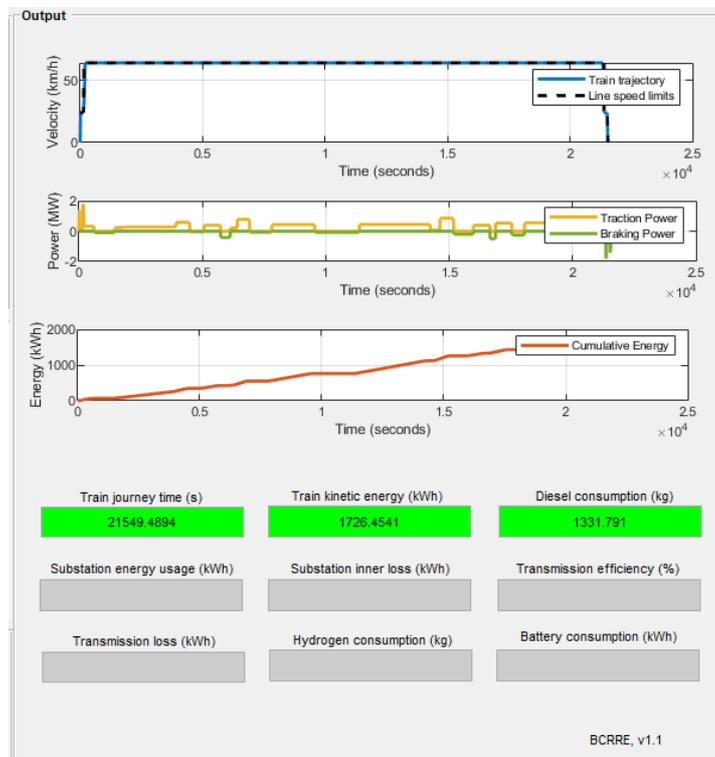
Figure B.5: Simulation output for the Mwanza – Tabora section, using the diesel only train
