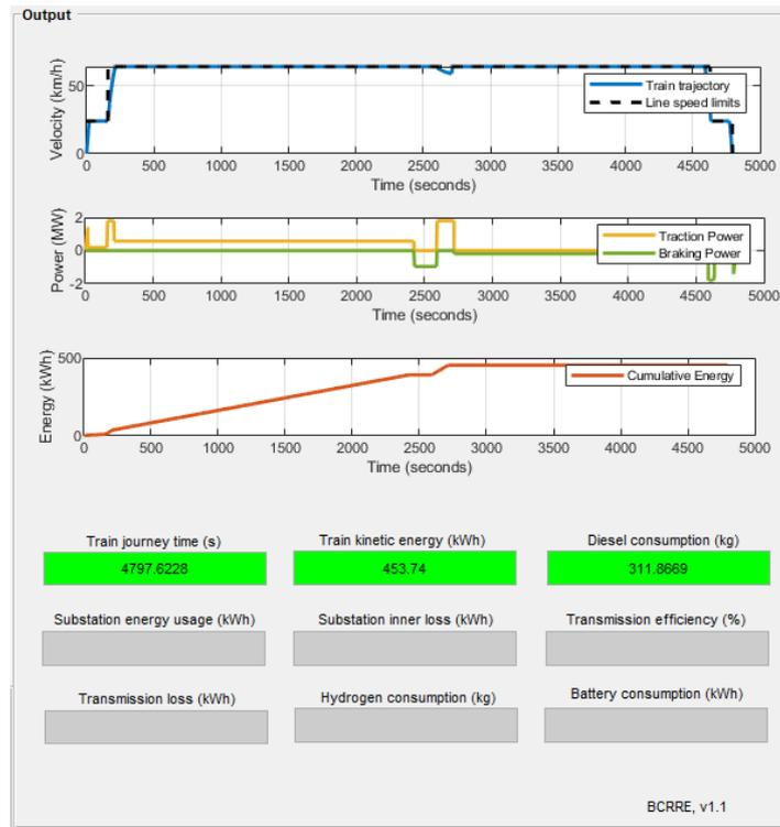
Figure B.2: Simulation output for the Mahundi Jn. – Tabora section, using the diesel only train
