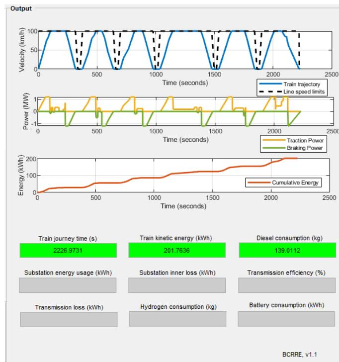
The route profile and STS results for the medium detail Google Earth map are shown in Figure C.8 and C.9 respectively. Note that this is smoother than the detailed Google Earth model but the results are similar.
