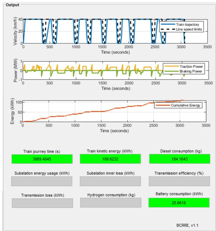
In addition, a battery-only ULR option was modelled assuming a 100 kWh battery per vehicle, to give a total of 500 kWh of storage and the same total power output of 840 kW. Figure 15 shows the results for this battery train.
