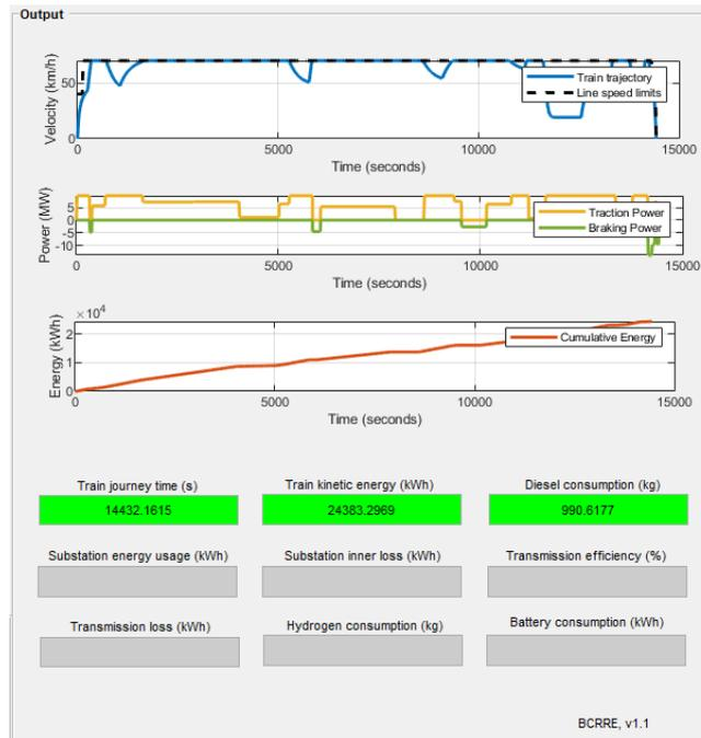
As can be seen in the figures above (i.e. Figure 20 and Figure 21), not only does the loaded train use 121.4 l more diesel than the empty one, but it also takes 1441 seconds (24.02 minutes) longer to complete the journey. Therefore, we can conclude that the train mass has a significant impact.
