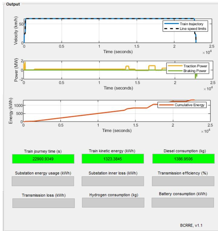
Figure 37: Simulation output for the Kigoma – Tabora section, using the diesel hybrid train
