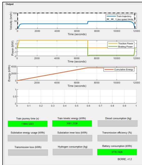
Figure 5: Simulation results for the loaded train on the hypothetical 120 km route
