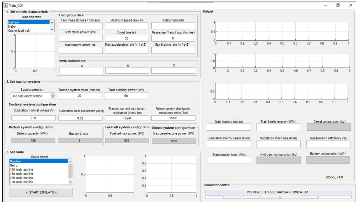
Section 1 of the GUI concerns vehicle characteristics. There are several default options, or one can customise their own train, using the train properties in this section, including:
