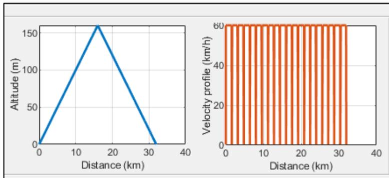
The simulation results are shown in Figure 13. It should be noted that the mass of the train was increased to 32 tonnes. The simulated mass includes a 10 tonne allowance for passengers and extra traction system equipment over the tare weight of the base diesel powered unit that was used as a benchmark. The Davis equation has been calculated to be  $R = 0.9 + 0.018V + 0.0041V^2$ . Simulation results are shown in Figure 14.
