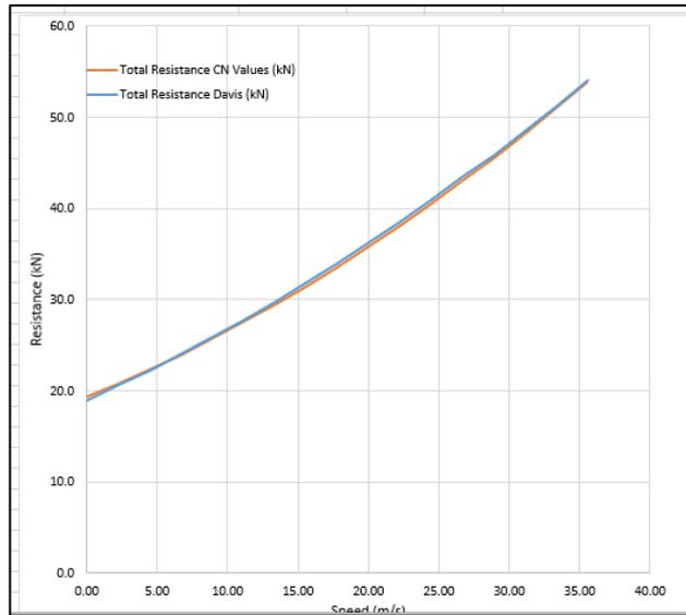
**Figure A.4: Comparison of the Canadian National resistance calculation (orange) with the approximated Davis equation curve from equation A.2 (blue) (empty freight train)**
