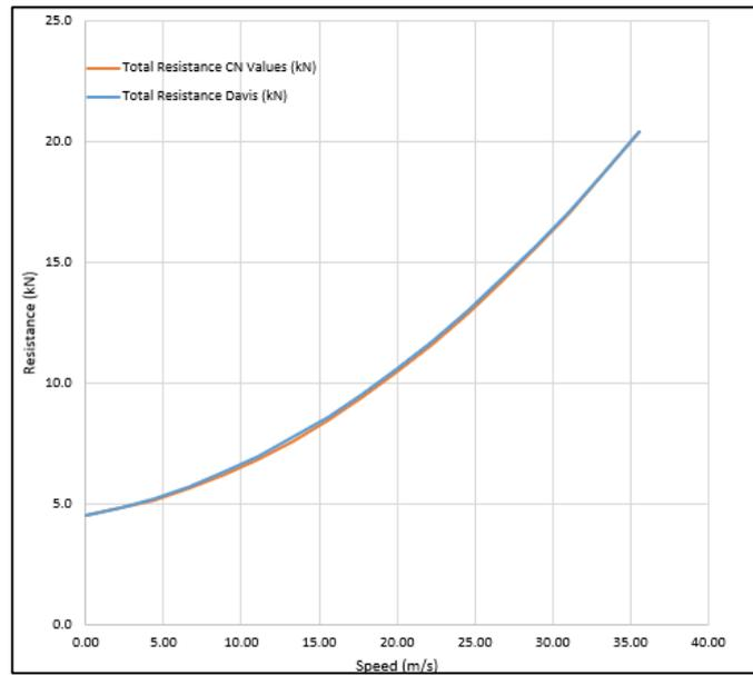
Figure A.10: Comparison of the Canadian National resistance calculation (orange) with the approximated Davis equation curve from equation A.5 (blue) (loaded shunter train)
