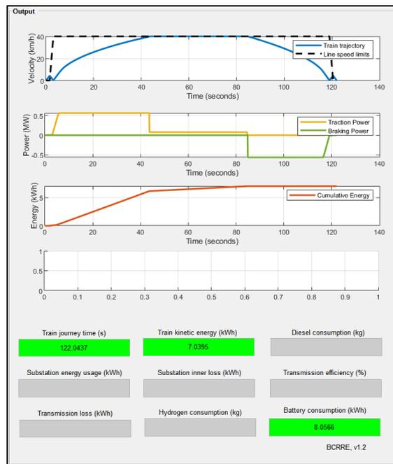
Figure 11: Simulation results for the empty shunter train on the hypothetical 1 km route
