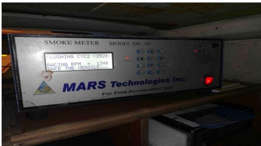
**Figure 6:** Emissions testing equipment: Smoke Meter Model SM 05; Acceleration tests provided by Mars Technologies Inc
