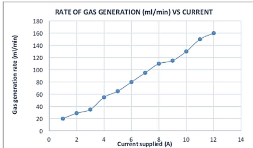
**Figure 3:** Gas generations with different inputs
