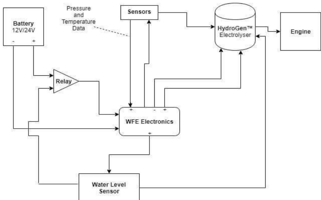
**Figure 5:** WFE electronic control unit
