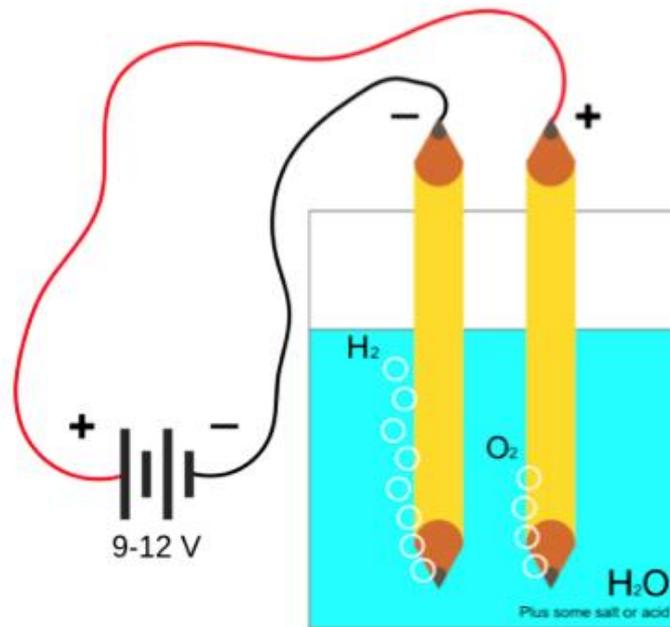
**Figure 1:** A simple electrolysis experiment
