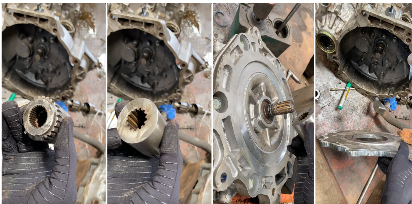
Figure 13: Modifications to adapt the electric motor to the gearbox
