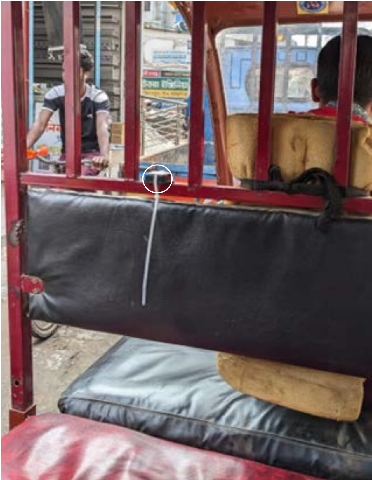
Figure 14 IMU Sensors Attached to Seats (Marked by the white circle)
