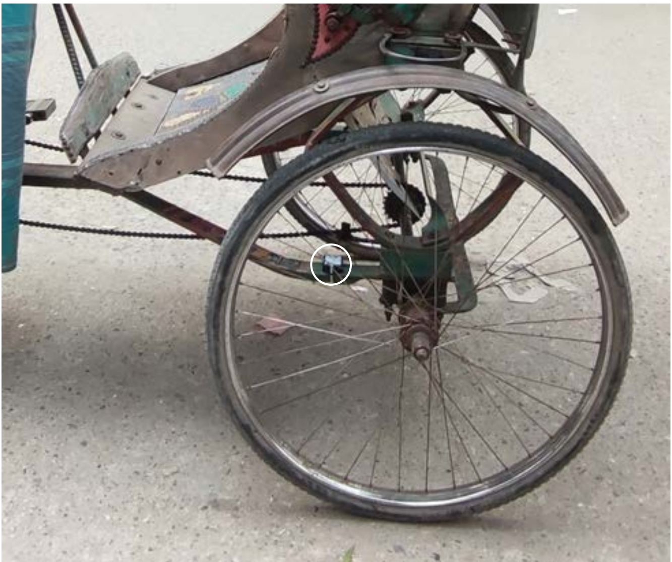
Figure 13 IMU Sensors Attached to Rickshaw Frame (Marked by the white circle)
