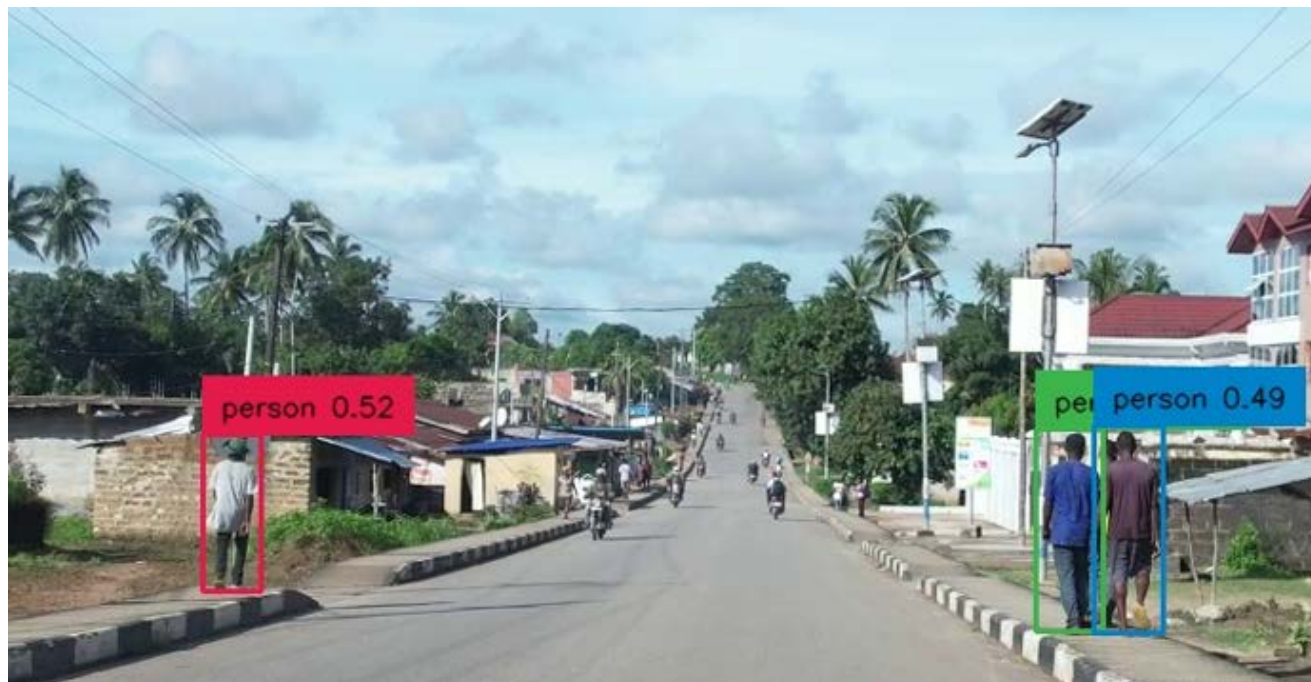
Figure 22: Example of “short sightedness” of the object detector, as it is unable to detect any of the motorcycles which are obvious to a human viewer
