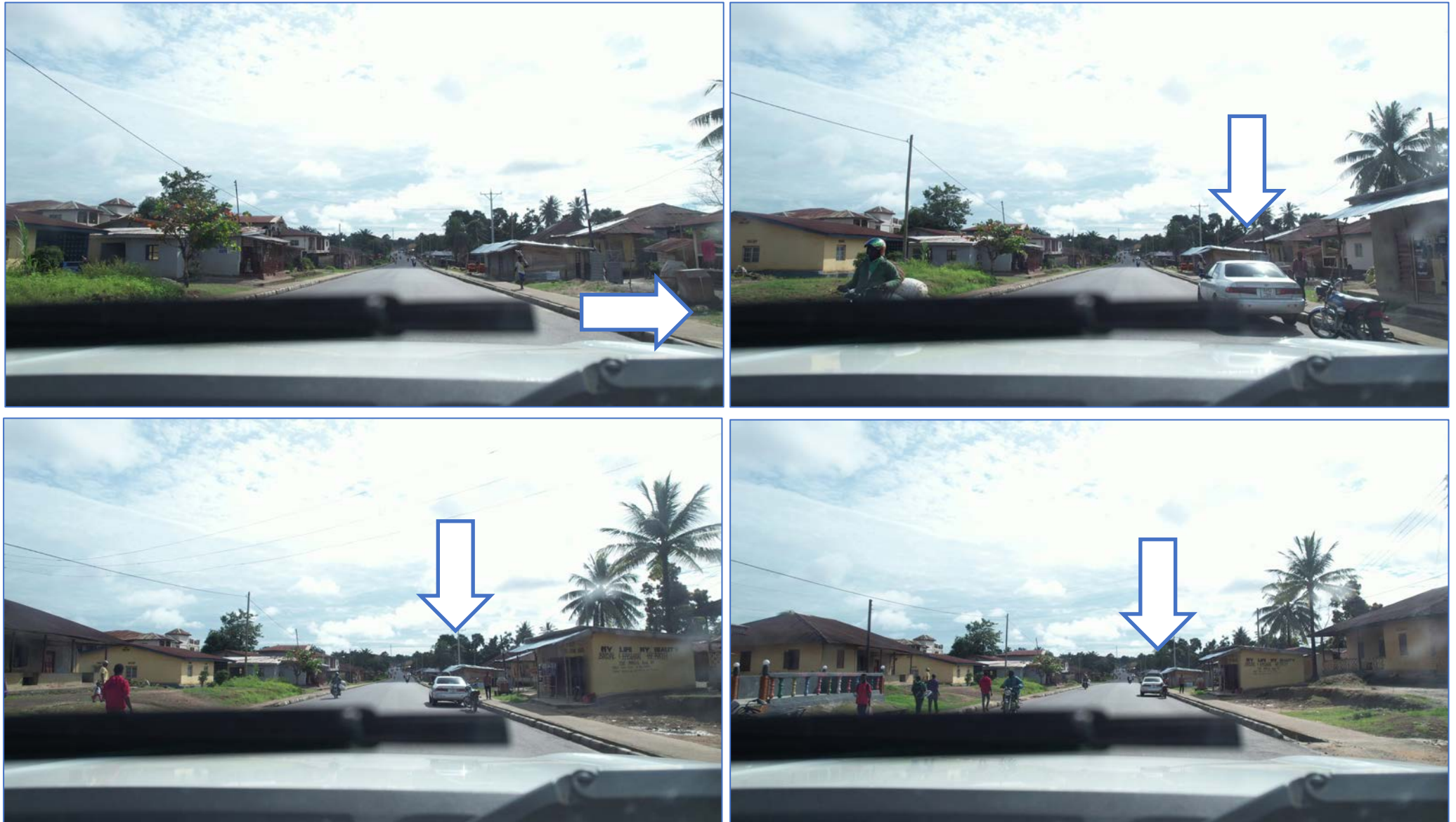
Figure 19: The position of a parked car relative to the centre of the image changes as the camera moves closer. The same behaviour is seen in moving cars, so this method cannot be used to distinguish moving and parked cars.
