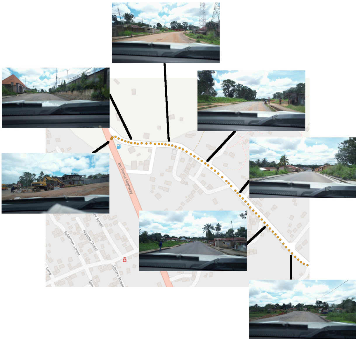
Figure 10: Example of frame extraction (please note this is for demonstration only – for use in the tool, one frame was extracted for every GPS observation, rather than every tenth observation as shown in this diagram)
