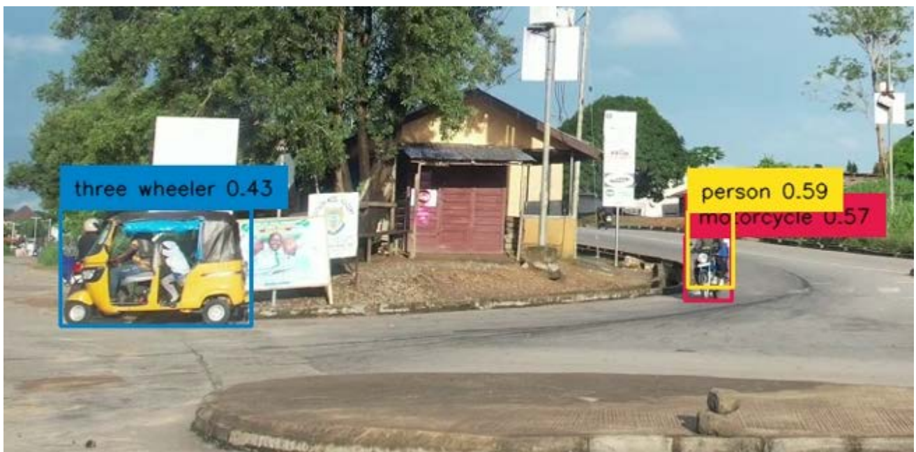
Figure 13: Detection of a keke (three wheeler) and a motorcycle
