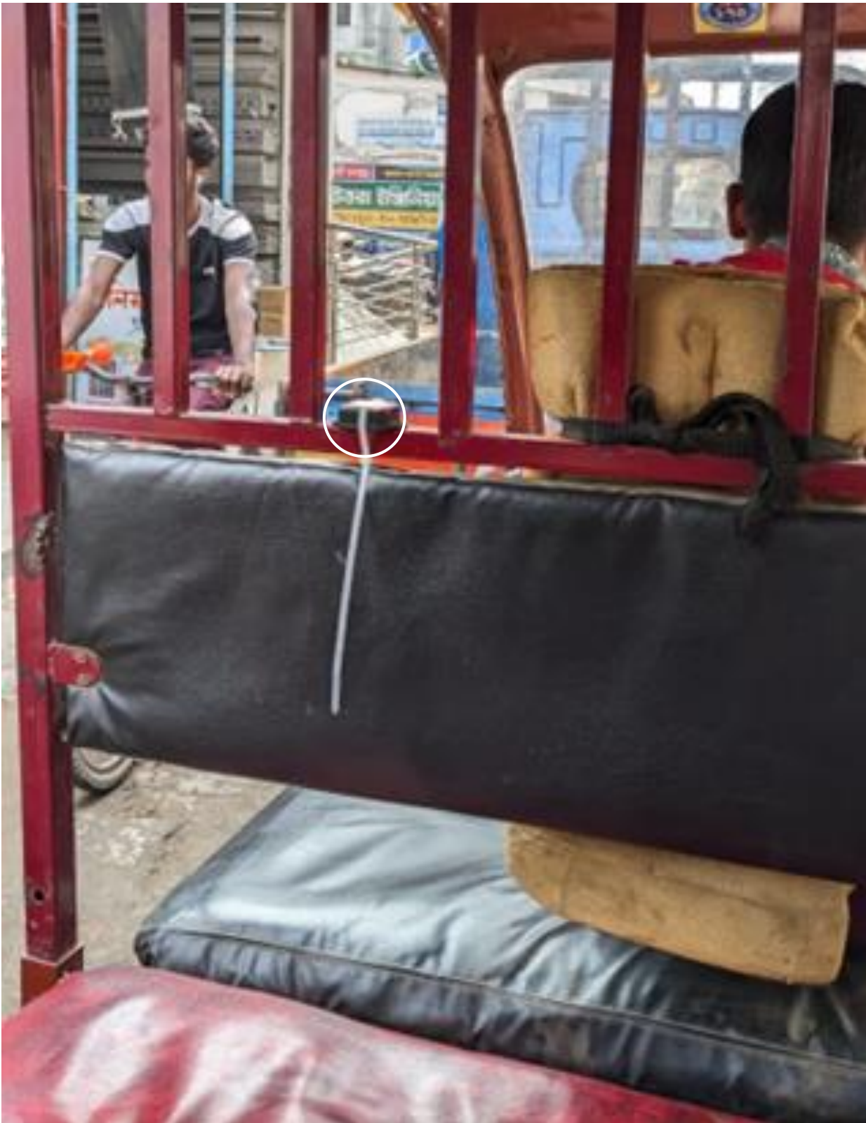
Figure 14: IMU Sensors attached to seats (marked by white circle)
