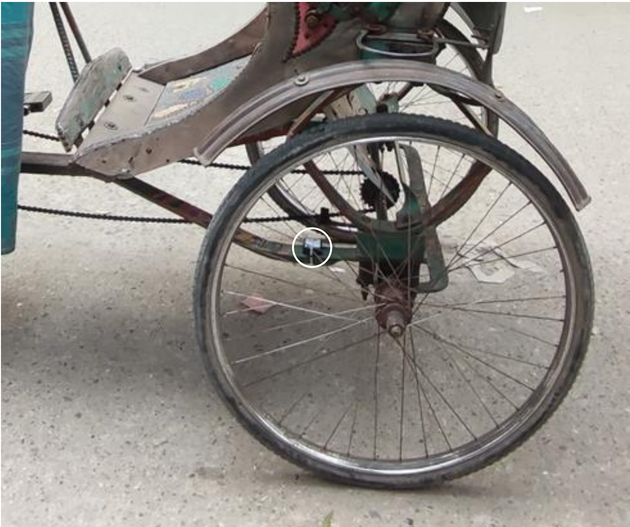
Figure 13: IMU Sensors Attached to Rickshaw Frame (Marked by White Circle)
