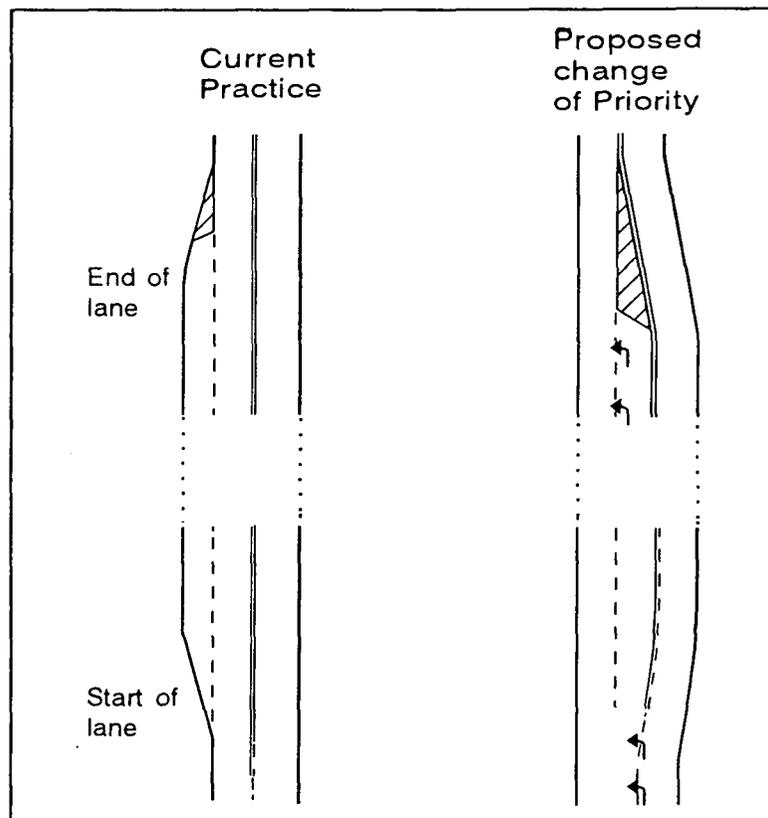
**Fig. 8 Proposed change of priority for ends of crawler lanes**
