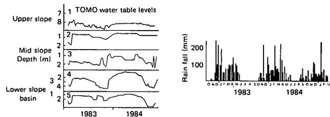
Fig. 3: Standpipe groundwater levels
