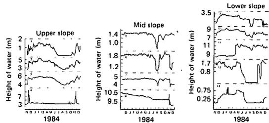
Fig 8: Piezometer levels at one site
