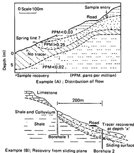
Fig 7: Results from dye tracer tests
