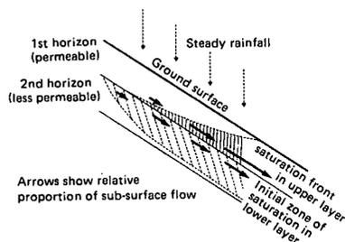
Fig 4: Slope saturation model. (Whipkey et.al)
