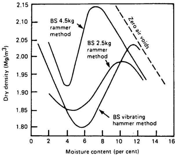
Fig. 5 Dry density/moisture content relationship for road base gravel (pilot scale trials)
