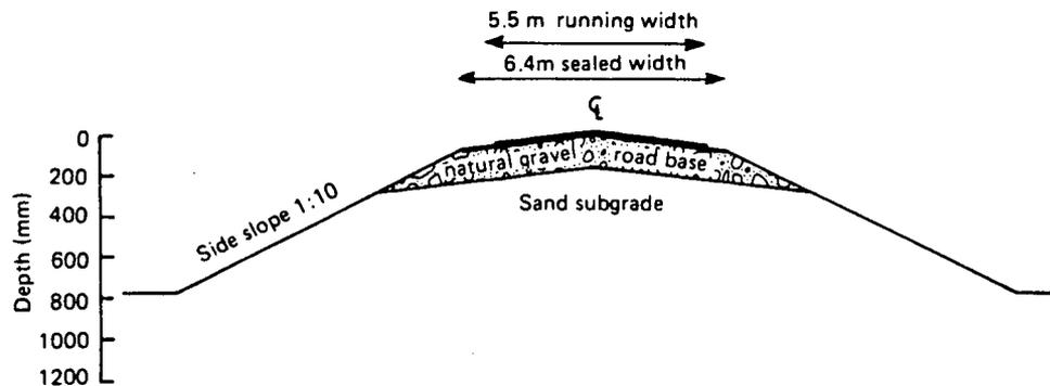
Fig. 7 Layout of full scale trials
