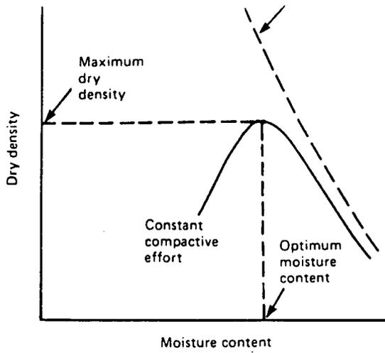
Fig. 1 Conventional compaction curve
