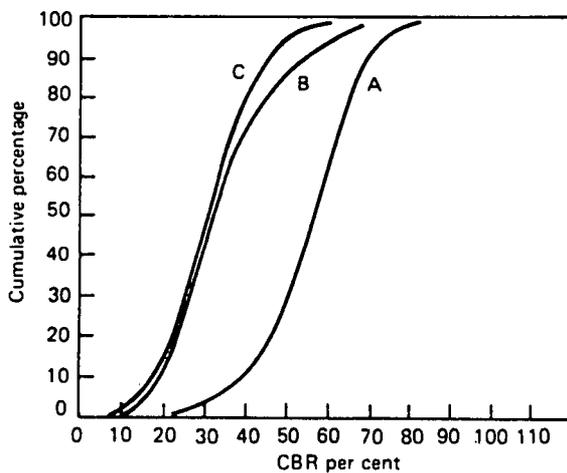
Fig. 8 Distribution of subgrade CBR's (DCP method)
