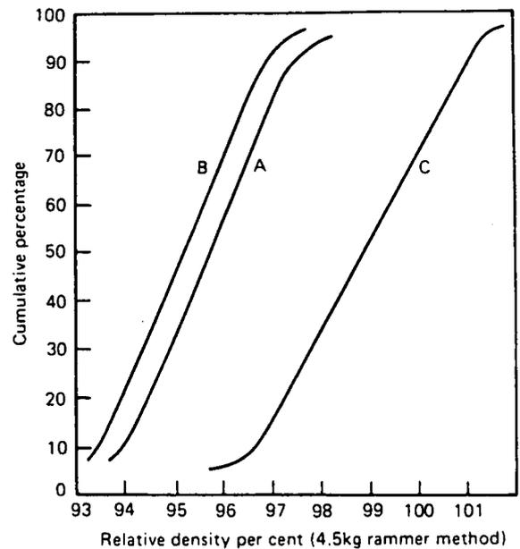
Fig.10 Distribution of field densities at construction
