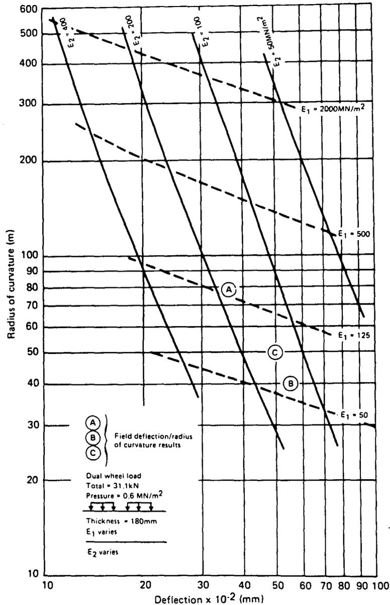
Fig. 15 Relationship between radius of curvature and deflection
