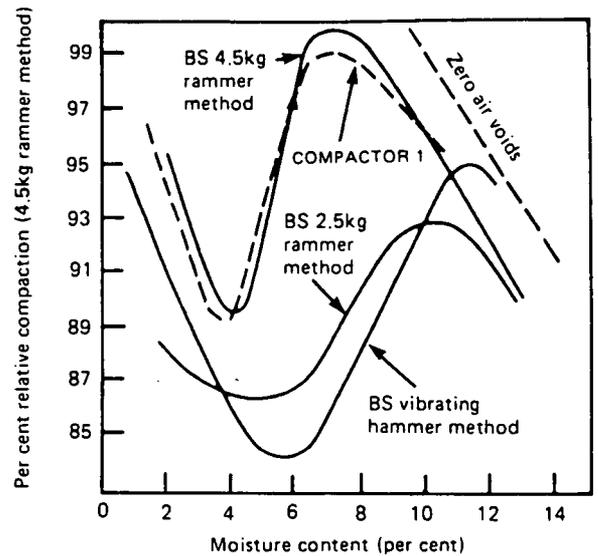
Fig. 6 Field dry density/moisture content relationship relative to laboratory methods, for compactor 1.
