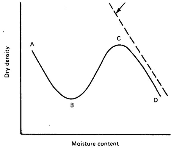
Fig. 2 Extended compaction curve for low moisture contents
