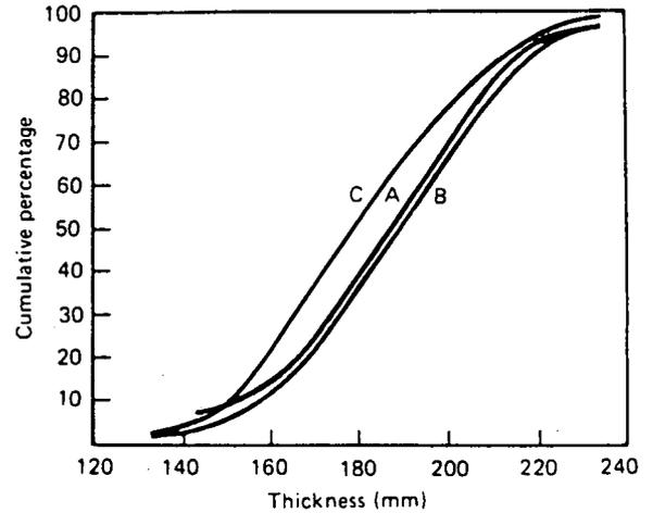
Fig. 13 Distribution of roadbase thickness
