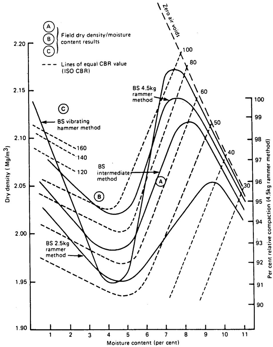
Fig. 11 Laboratory CBR/dry density/moisture content relationship for road base gravel (full scale trial) with field results
