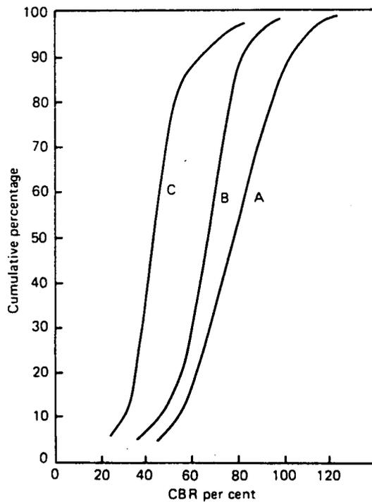
Fig. 12 Distribution of roadbase strength at construction (Clegg Impact Hammer)
