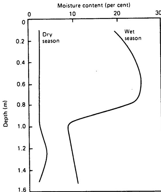
Fig. 14 Open ground moisture content profile
