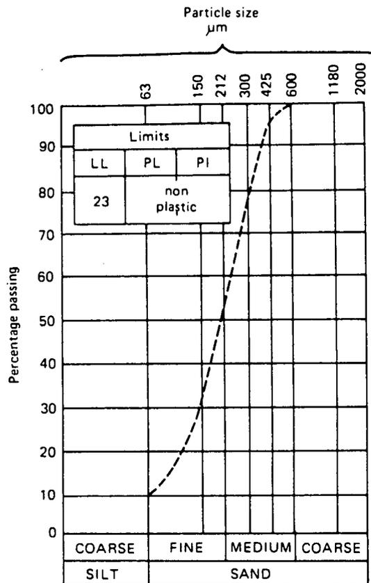
Fig. 9 Particle size distribution of subgrade material
