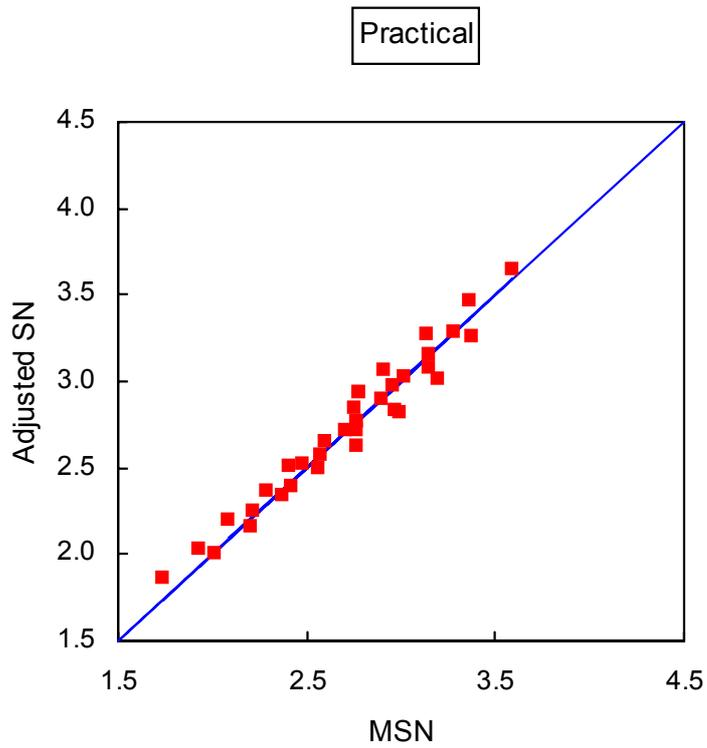
Figure 2. Comparison of the new adjusted method to the original method for typical pavement structures (Road Note 31 Chart 1)
