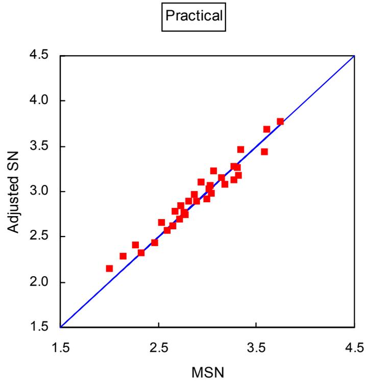
Figure 3. Comparison of the new adjusted method to the original method for typical pavement structures (Road Note 31 Chart 8)
