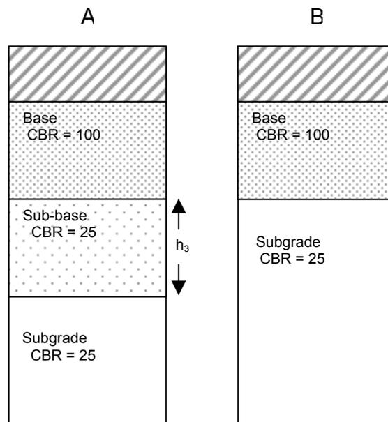
Figure 1 Identical pavements, different structural numbers
