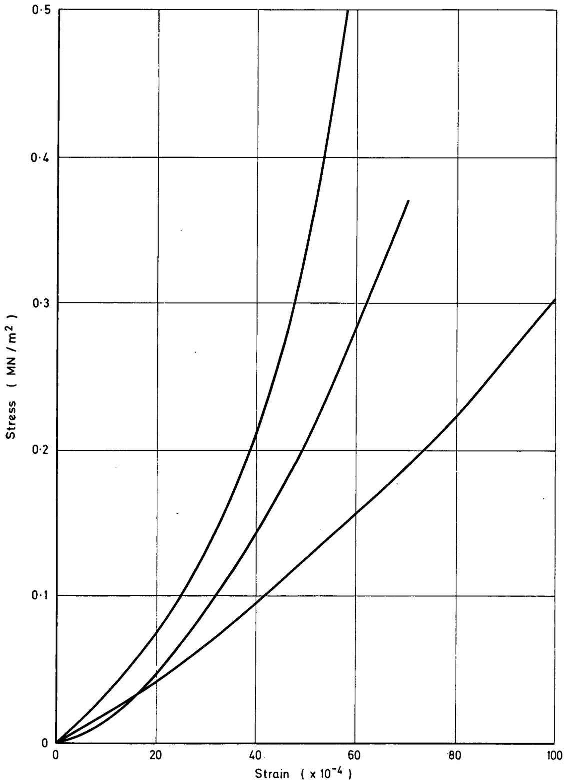
Fig. 8 TENSILE STRESS-STRAIN CURVES FOR SPECIMENS SAWN FROM THE PAVEMENT AT ROMPIN ( HOLE 3 ), MALAYSIA.
