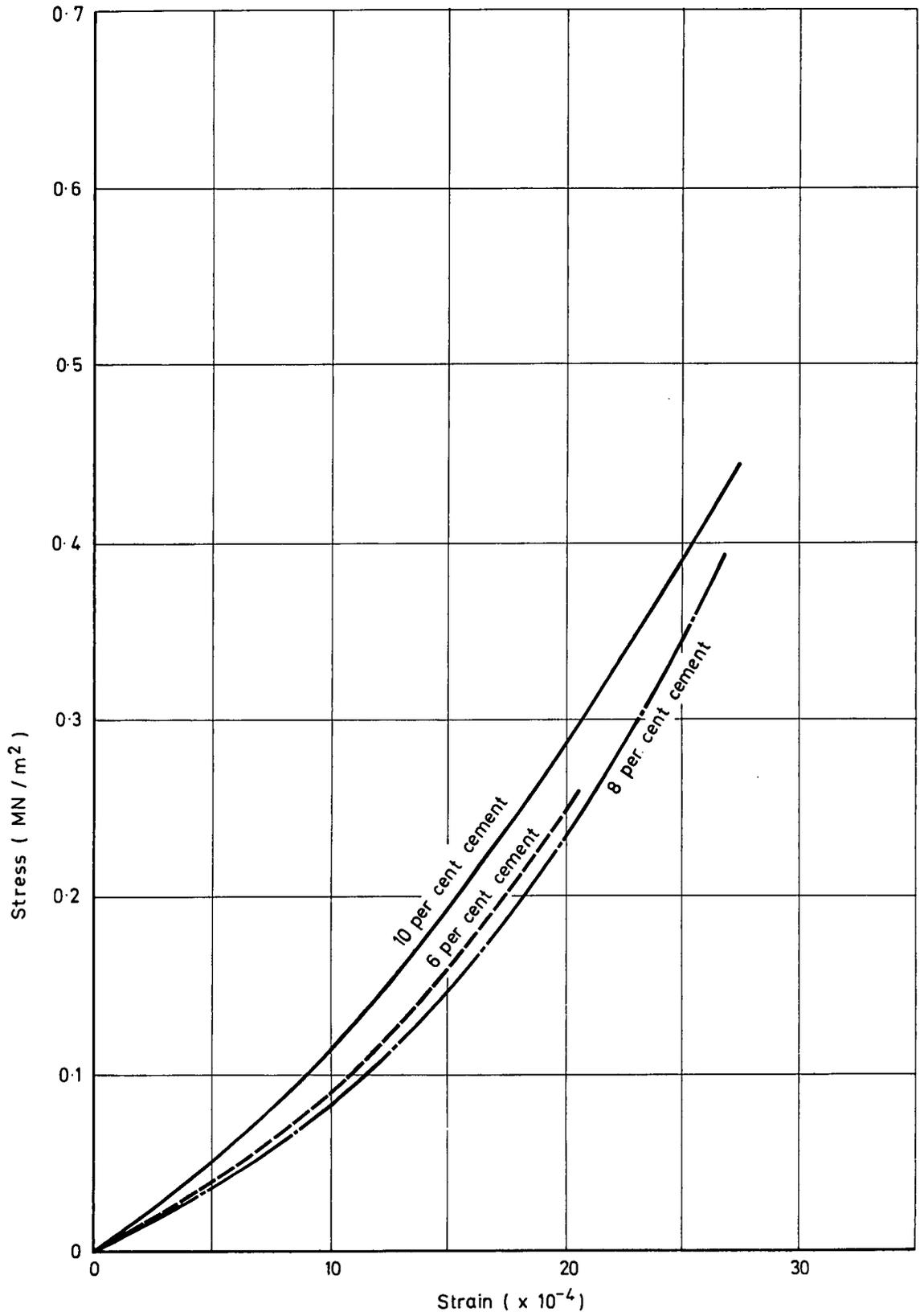
Fig. 6a AVERAGE TENSILE STRESS-STRAIN CURVES FOR CEMENT-STABILISED HARMONDSWORTH BRICKEARTH MOULDED AT 15 PER CENT MOISTURE CONTENT
