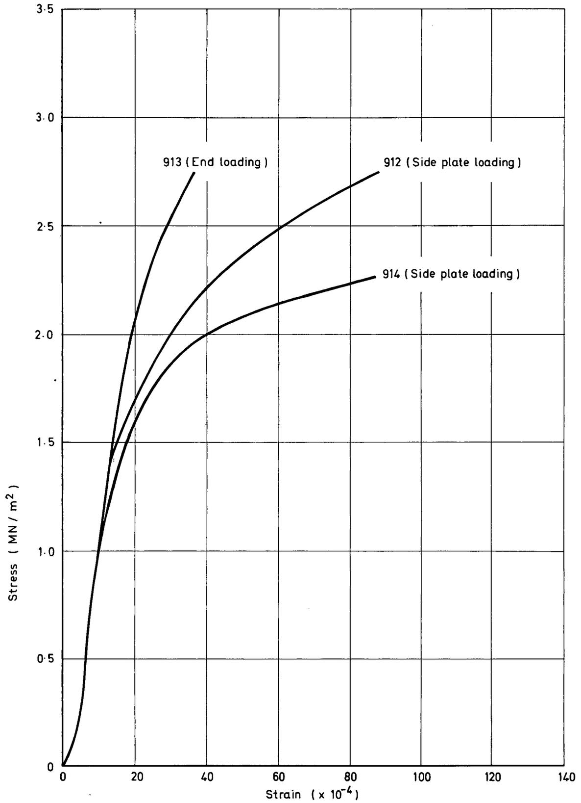
Fig. 5 COMPRESSIVE STRESS-STRAIN CURVES SHOWING THE EFFECT OF SIDE PLATES CEMENTED TO THE ENDS OF THE SPECIMEN
