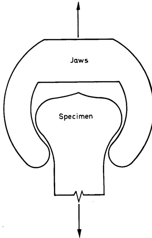
Fig. 1 TENSILE SPECIMEN LOADED THROUGH GRIPPING JAWS
