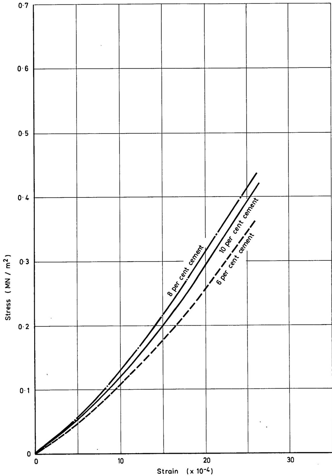
Fig. 6b AVERAGE TENSILE STRESS-STRAIN CURVES FOR CEMENT-STABILISED HARMONDSWORTH BRICKEARTH MOULDED AT 17 PER CENT MOISTURE CONTENT
