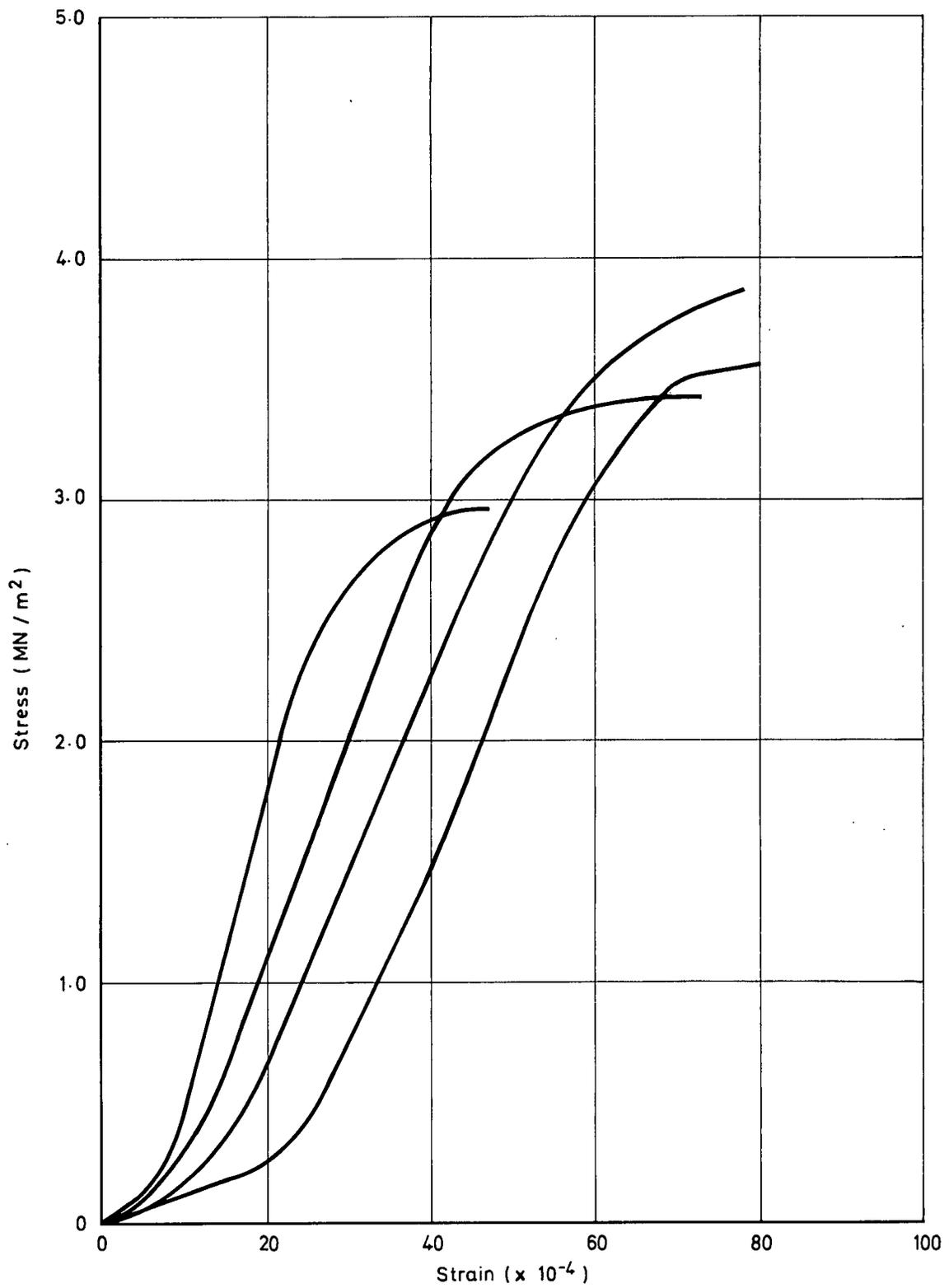
Fig.9 COMPRESSIVE STRESS-STRAIN CURVES FOR SPECIMENS SAWN FROM THE PAVEMENT AT ROMPIN ( HOLE 3) MALAYSIA
