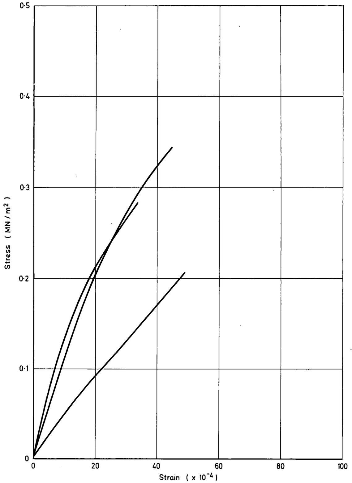
Fig. 10 TENSILE STRESS-STRAIN CURVES FOR SPECIMENS SAWN FROM THE PAVEMENT AT ROMPIN ( HOLE 5/6 ), MALAYSIA.
