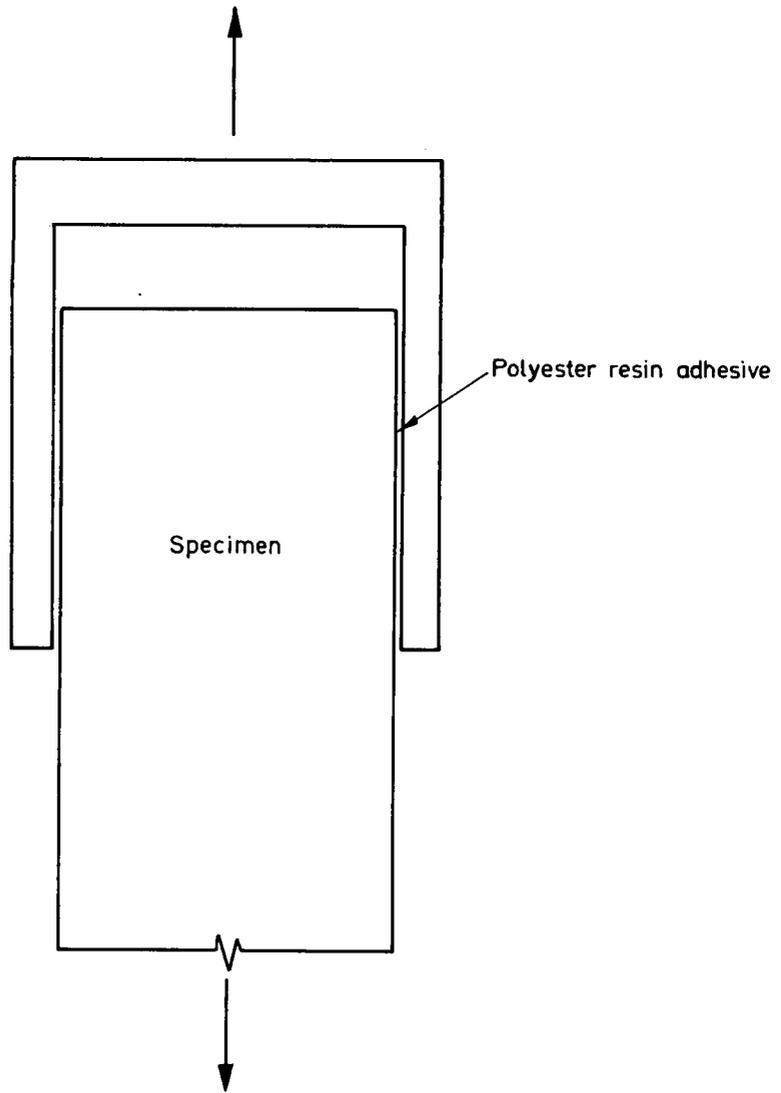
Fig.3 SCHEMATIC ARRANGEMENT OF TENSILE SPECIMEN LOADED THROUGH PLATES CEMENTED TO THE SIDES OF THE SPECIMEN AT EACH END
