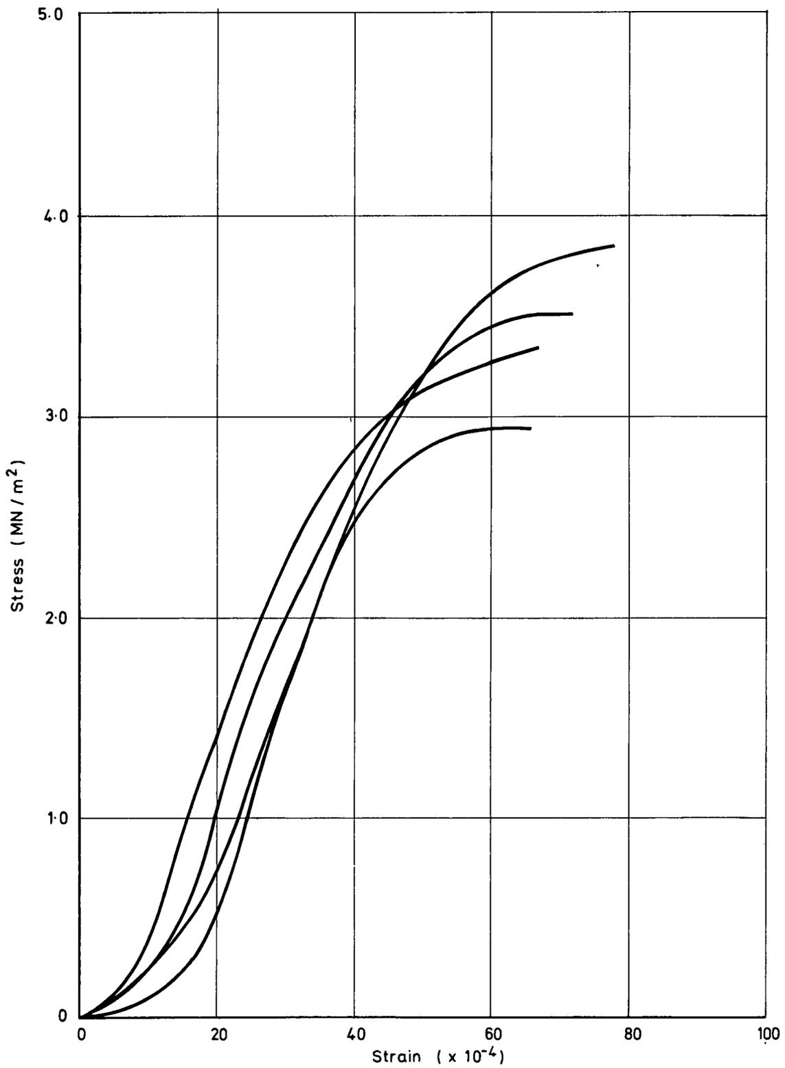
Fig.11 COMPRESSIVE STRESS-STRAIN CURVES FOR SPECIMENS SAWN FROM THE PAVEMENT AT ROMPIN ( HOLE 5/6 ) MALAYSIA
