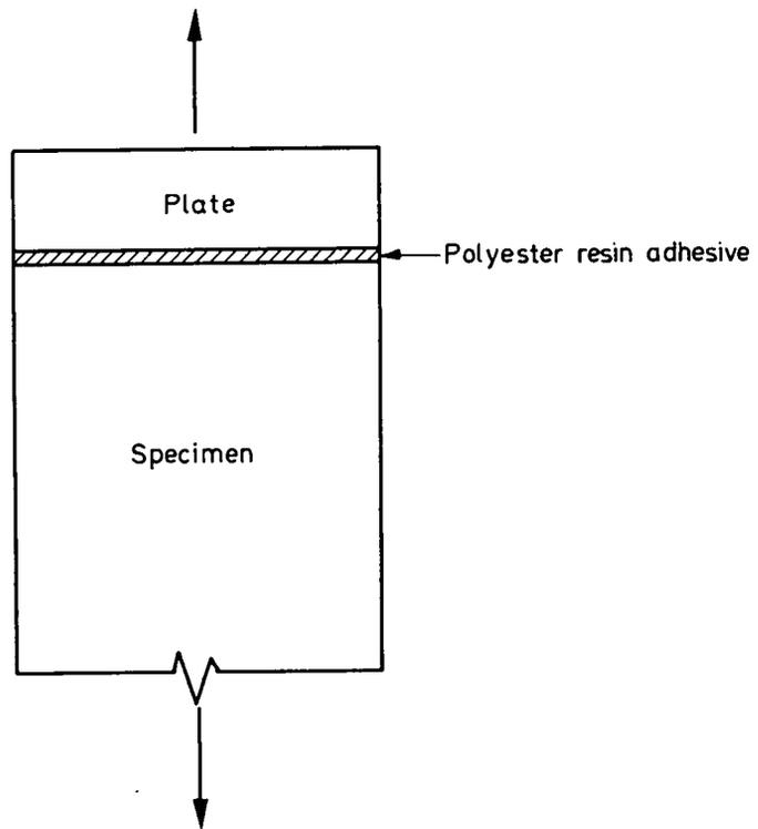
Fig. 2 TENSILE SPECIMEN LOADED THROUGH PLATES CEMENTED TO ITS ENDS
