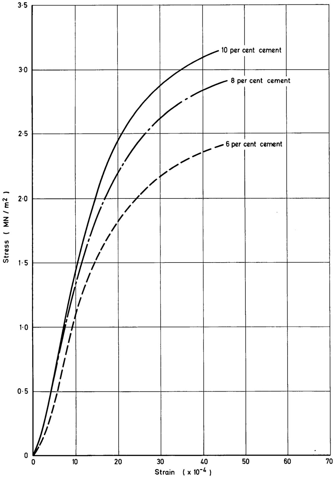
Fig. 7b AVERAGE COMPRESSIVE STRESS - STRAIN CURVES FOR CEMENT - STABILISED
