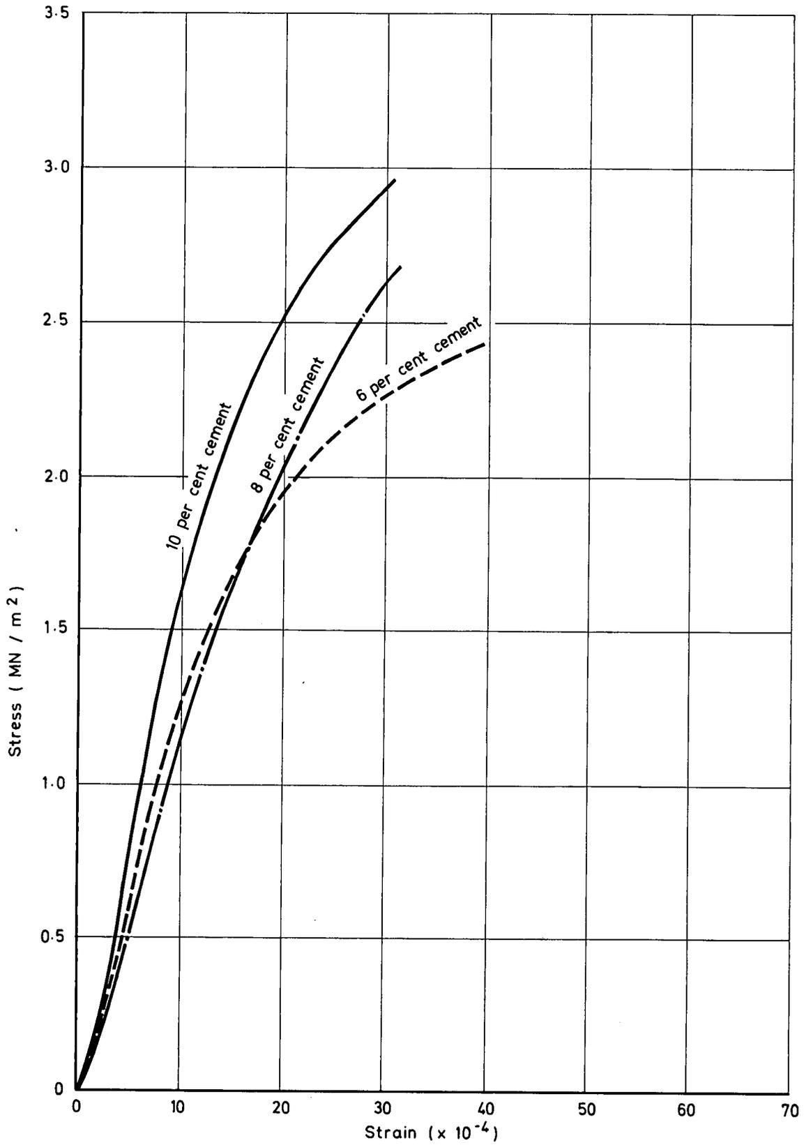
Fig.7a AVERAGE COMPRESSIVE STRESS - STRAIN CURVES FOR CEMENT - STABILISED HARMONDSWORTH BRICK EARTH MOULDED AT 15 PER CENT MOISTURE CONTENT.
